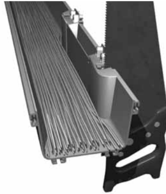
Fixture protects cables during cutting of sidewall
