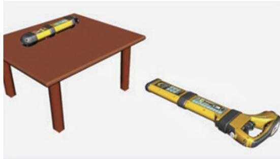
2. Switch on the transmitter and set the output to low. Set the receiver to 33 kHz Sonde mode. Set the sensitivity control so that the largest notch is pointing directly at the mode switch as below.
