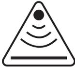
The overhead signal alert is triggered if vScan detects a significant signal radiating from above, for instance an overhead cable.
