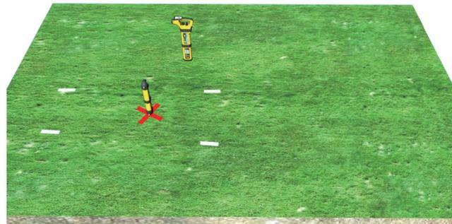
Note that, when the transmitter is positioned vertically as above, there is no signal induced directly below the transmitter. It is therefore necessary to move the transmitter approximately one meter to the side and repeat the locate exercise in case a service crossed directly below.
