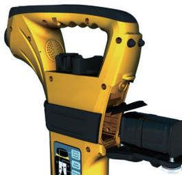
The battery can be charged in situ. Unscrew the ¼ turn fastener of the battery compartment (do not open the internal battery door). Align the red dot on the charger plug with the dot on the charging socket and connect together. Connect the supplied charger to the mains and switch on. The charging LED on the charger will illuminate red until the batteries are charged. The LED will then turn green indicating a full charge.
