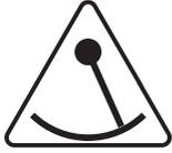
The swing alert will trigger if the angle of swing exceeds 30 degrees from the vertical. No alarm will be activated if the angle is more than 65 degrees from the vertical as it will be assumed that the locator is not in use at this time.
