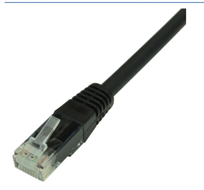
High Quality Cat 6 UTP Patch Lead Wired 258A (T568B) to 50 Micron Gold Plated RJ45 connectors. Each cable is supplied with fitted strain relief Boots for added protection. All cables up to 5m are made using standard core cable with cables over this length using solid core cable, which although not so flexible are more robust.
