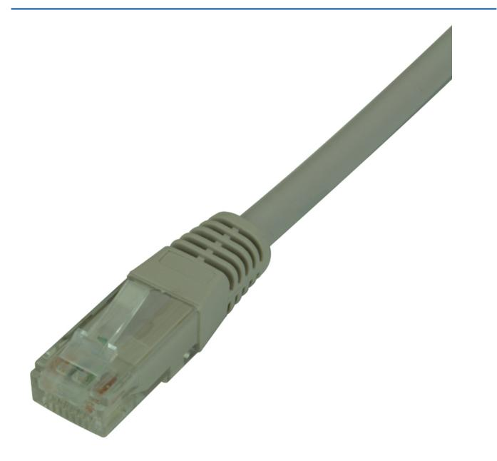
High Quality Cat 5e UTP Patch Lead Wired 258A (T568B) to 50 Micron Gold Plated RJ45 connectors. Each cable is supplied with fitted strain relief Boots for added protection. All cables up to 5m are made using standard core cable with cables over this length using solid core cable, which although not so flexible are more robust.
