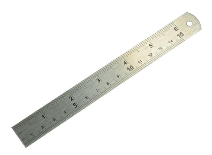
A precision rule manufactured from hardened stainless steel. The steel rule benefits from clear black graduation markings in metric of 0.5mm, 1mm, 0.5cm, 1cm and imperial markings of 1/64", 1/50", 1/32", 1/20", 1/16", 1/10", 1/2".
