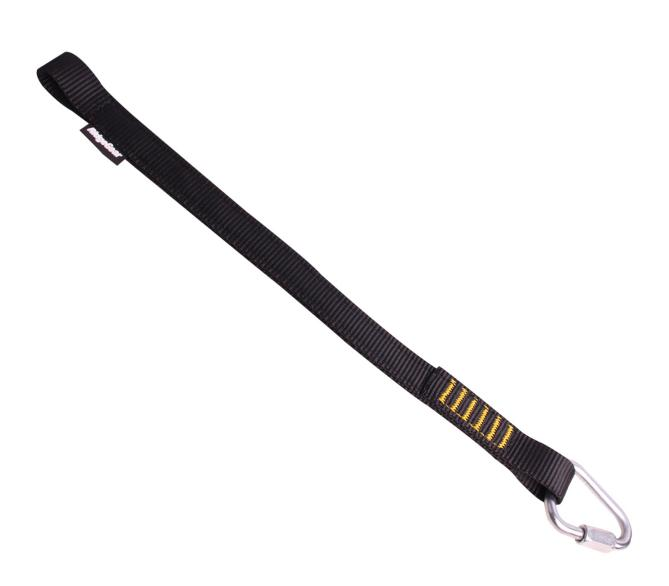
The RGL4 is used as an extension strop fitted to the rear D ring of a full body harness. It features a sewn eye on the free end allowing the operative to independently connect themselves to a fall arrest block by extending the attachment point on the harness and bringing it into the field of vision.
