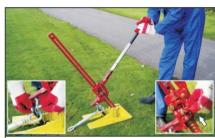
10. Connect the jack to the top eye of the anchor using the shackle and with the jack's direction lever in the 'up' position, operate the jack to apply a load to the anchor.
