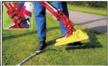
12. Move the jack's direction lever to the 'down' position and operate the jack to lower it. Caution! Once the load has been released, the jack will drop to its lowest position. Disconnect the jack from the anchor. The anchor can now be put into service.
