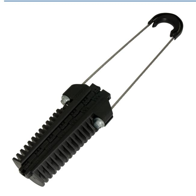
These anchoring clamps are designed for the dead-ending of FTTH aerial round cables from 5mm up to 6mm, with reinforced outer sheath.
