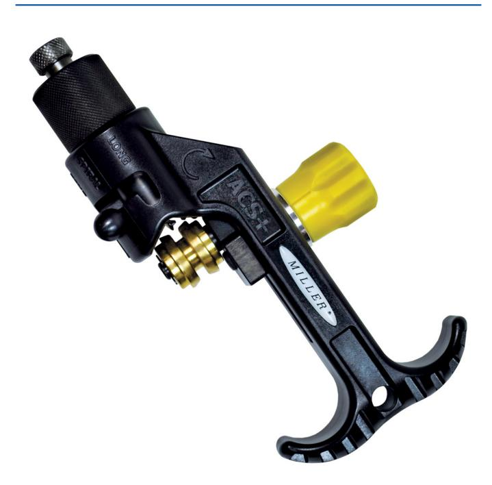
Designed for use on armoured fibre feeder, central tube & stranded loose tube fibre optic cables, as well as various other non-fibre armoured cables, the ACS Plus easily cuts through the polyethylene jacket and corrugated copper, steel or aluminium armour layer in one smooth step.
