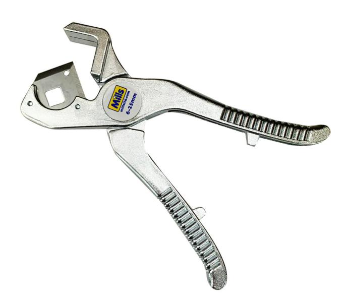
Diecast zinc alloy bodied cutter fitted with reversible hardened and tempered replaceable steel blade. Also suitable for cutting rubber hose and pipe. Length 190mm.
