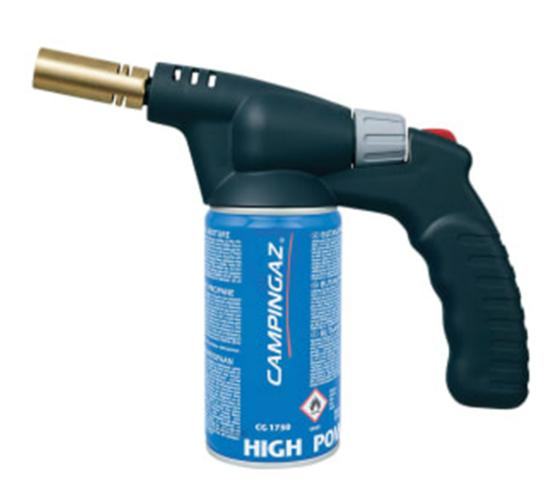
This auto blowlamp has a highly ergonomic, shock-resistant polypropylene handle for comfortable use. With Piezo automatic ignition, it is extremely easy to light. The brass burner produces a flame which allows fine adjustment via a nozzle. It can be operated off either the Campingaz® CG1750 or CG3500 valve cartridges.
