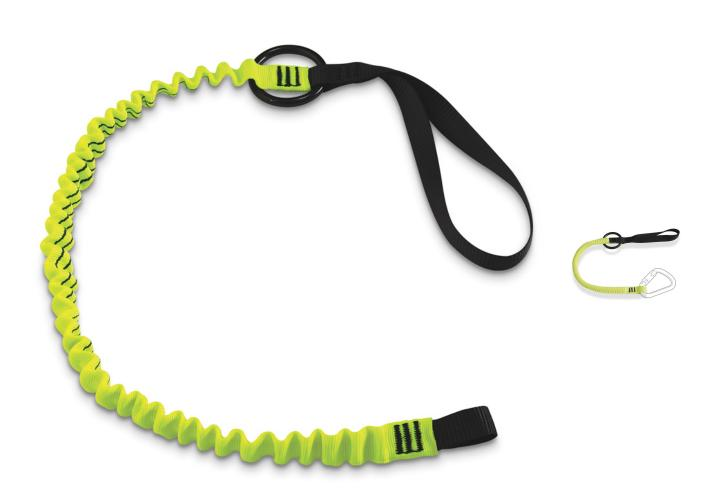
The RTLE3 is an elasticated tool lanyard with a choke loop for tool attachment and an 'O' ring for retention of a tool. It is suitable for tools up to 5kg in weight
