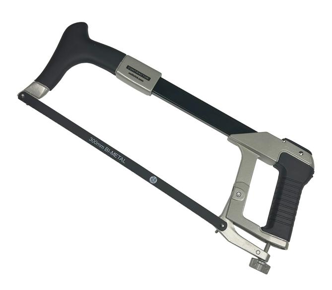
CONTRACTOR Hacksaw for use with 12" (300mm) blades, with soft grip handle. Manufactured from enamelled aluminium with two sets of blade spigots, which allows the hacksaw to be used for straight and 45 degree cutting. the hacksaw is supplied complete with 24TPI HSS blade.
