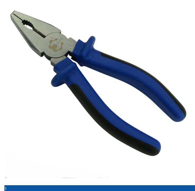
ECO-TOOLS engineering grade chrome vanadium combination plier with induction hardened cutting edge, and gripping zones for flat and round material. The plier also benefits from a bi material comfort grip for higher leverage and repetitive use- total length 6" (150mm)
