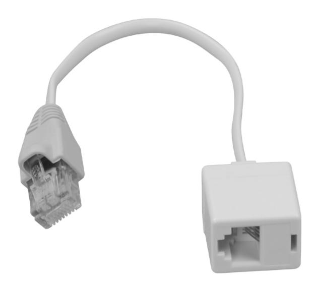
An adaptor to enable an RJ11 plug to be connected to an RJ45 socket. Designed specifically for use with Tone and Probe cable tracing kits that commonly have RJ11 plugs on the tone oscillators to prevent the damage that often occurs when an RJ11 plug is inserted directly into an RJ45 socket.
