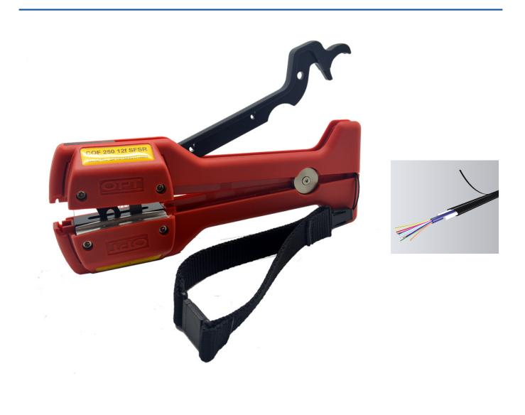
The OPT stripper has a profiled cassette that makes two longitudinal parallel slits in the sheath on one side of a COF250, SST Drop Cable or 12f Flat Drop Wire Cable (typically as supplied by Corning ). One cassette contains two rotary blades which cuts through the outer sheath to enable a portion of the sheath to be 'peeled' away and expose the cable element.
