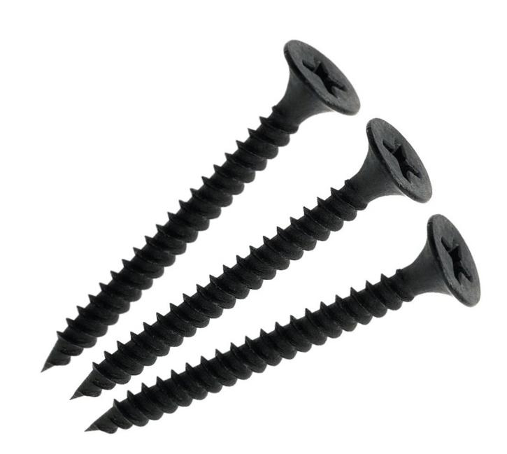
Countersunk Phillips drywall screws are ideal for fastening dry lining and plasterboard to studwork. These screws have a twin thread and sharp point for fast installation and benefit from a black phosphate finish for durability.
