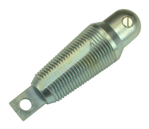
Subduct pulling eye, also known as a Carrot or Grip Threaded, with clevis pin and eye to attach draw rope etc Units are tapered and threaded. Zinc plated
