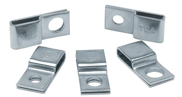
Suitable for the secure fixing of cables, tubing, conduits and pipes within the most arduous of environments. Providing a complete fastening and fixing solution when used in conjunction with stainless steel ties up to 10.0 mm width. Made from Grade 316 Stainless Steel (SS316). Available with three different hole sizes.
