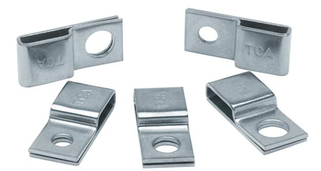
Suitable for the secure fixing of cables, tubing, conduits and pipes within the most arduous of environments. Providing a complete fastening and fixing solution when used in conjunction with stainless steel ties up to 10.0 mm width. Made from Grade 316 Stainless Steel (SS316). Available with three different hole sizes.
