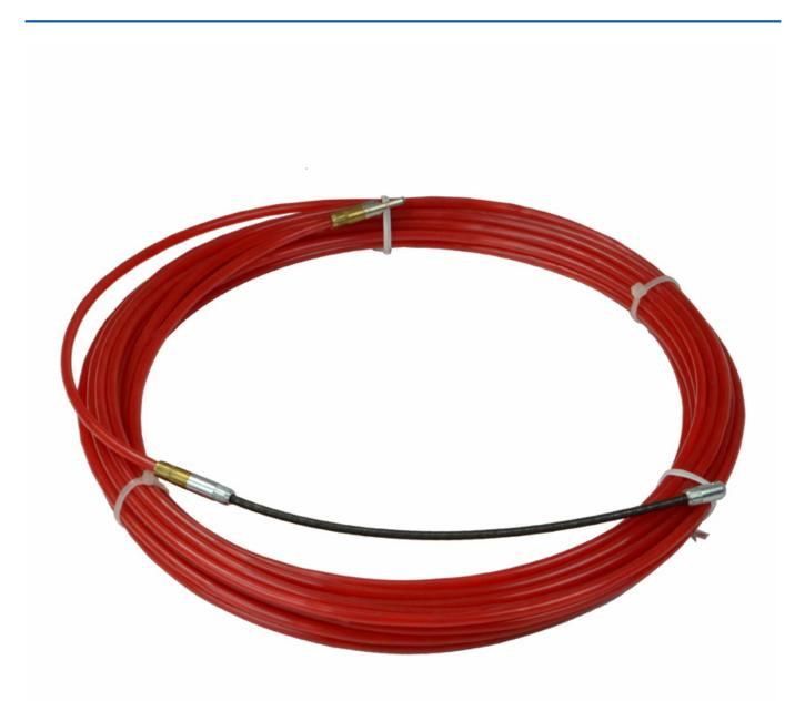
Non-conductive 4mm nylon construction for use in telecom, electrical, wall and floor conduit. and designed for pulling cables through occupied duct and panel boxes. The draw tape has a breaking strain of 100Kg, a bend radius of 38MM and has a 150mm flexi end leader with pulling eye at one end of the rod.
