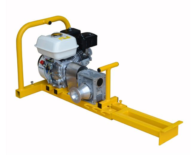
This lightweight capstan winch is designed for use over manholes, for simple cable pulling and cable recovery. Powered by a 5HP Honda Engine through a right angle gearbox, it has a pulling capacity of 1000kg using a 12mm diameter rope (recommended) via a 100mm diameter aluminium Diablo capstan at a rope speed of 18m per minute.
