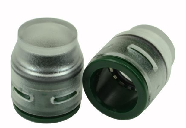
14mm Outside Diameter Microduct end cap to be used for sealing off microducts prior to installation or with C00-6697 Microduct Pressure Inflator Gauge and S83-6189 Air Flow Gauge Duct when conducting pressure checks prior to installation.
