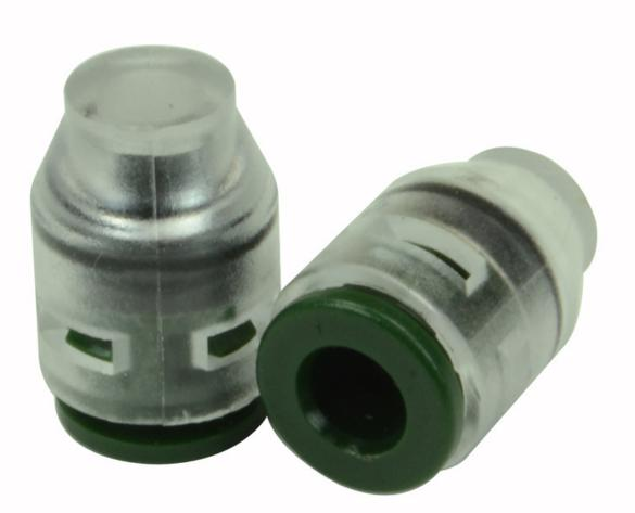
7mm Outside Diameter Microduct end cap to be used for sealing off microducts prior to installation or with C00-6697 Microduct Pressure Inflator Gauge and S83-6189 Air Flow Gauge Duct when conducting pressure checks prior to installation.
