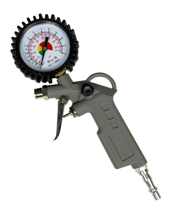
A simple air inflator for testing the integrity of blown fibre duct installations or micro duct pressure testing. The inflator can pressurise ducts up to 12 Bar. It is supplied with a standard PCL fitting, 8mm straight thread to tube adaptor and 400mm of 8mm duct as standard. This 8mm adaptor can be adapted to fit other tube diameters, by use of the reducing adaptors shown on this page. The inflator should be used in conjunction with end caps and the S83-6189 Air Flow Gauge.
