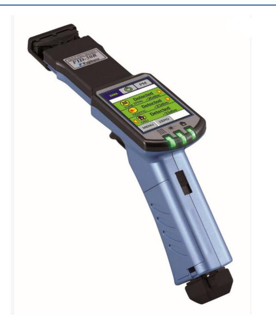
The FID-30R includes an optical power meter and succeeds the FID-25R. The fibre identifier, used for identifying the light power presence in optical fibres, includes three detecting functions: TONE, TRAFFIC, and ONU.
