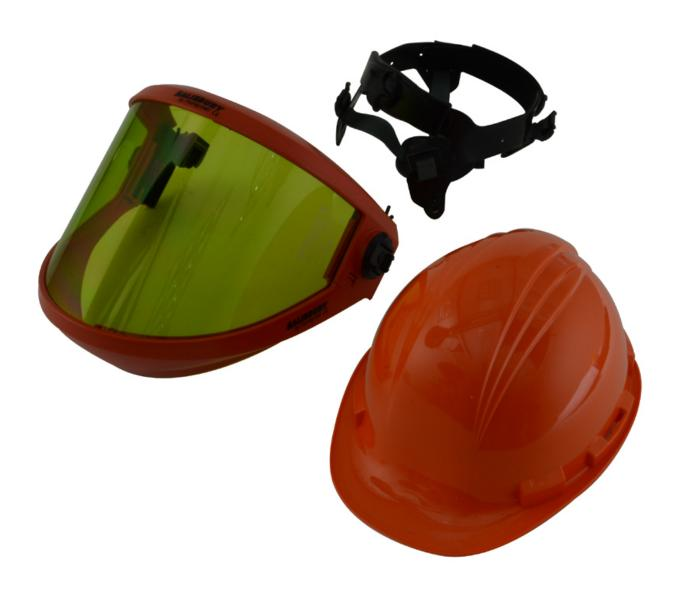
Features an Arc Rating of 12cal/ cm<sup>2</sup> (ATPV according to ASTM F2178) and utilises nanotechnology to provide a clearer, more transparent window for improved visibility. The faceshield unit includes ventilation ribs that allow a natural convection air flow through the top of the face shield. This reduces fogging of the visor, lowers CO<sup>2</sup> levels and improves comfort for the user. The assembly is also tested and certified to GS- T-29, Class 2.
