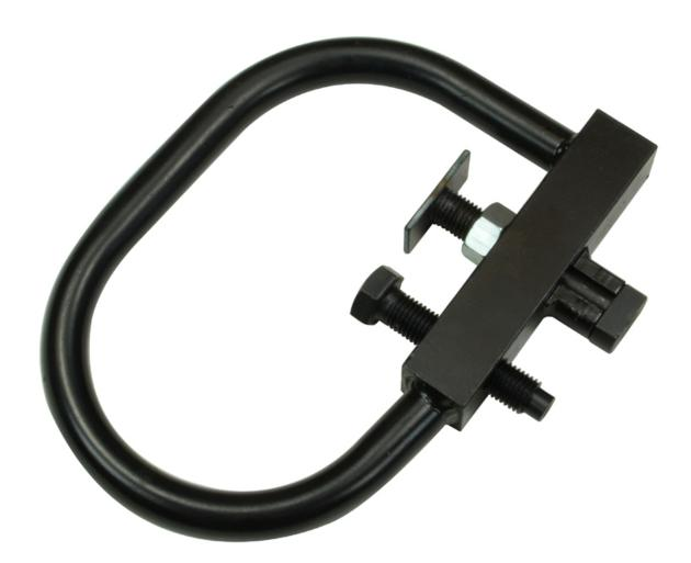
A steel tool for lifting E type and unit type covers of rectangular and square shape. The key is locked to the cover by an adjustable locking nut, then a jacking bolt is turned which bears against the frame to lift the cover. SWL 1 tonne
