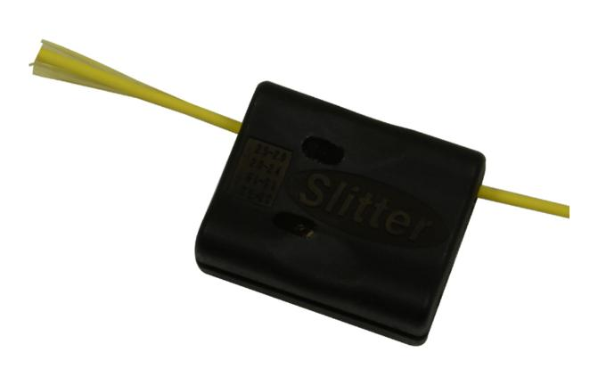
'The Slitter', Mid Span Fibre Access Stripper 1.5- 3.3mm- A simple and effective longitudinal sheath stripper tool for easy removal of the outer sheath of most fibres including loose tube with a diameter of 1.5mm to 3.3mm. Once the fibre has be placed in one of the 4 preset grooves, (1.5-1.9mm, 2.0-2.4mm, 2.5 -2.9mm and 3.0-3.3mm) the 'Slitter' can simply be pulled along the its length, slitting the outer sheath into two halves.
