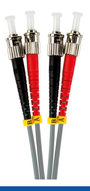
Duplex multimode OM1 62.5/125um fibre cable terminated at both ends with ST connectors. Length 3m
