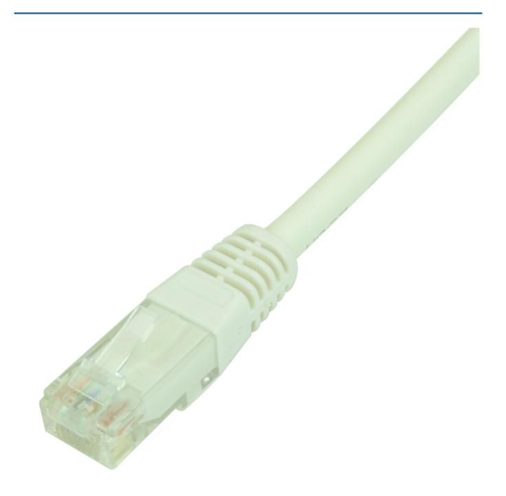
High Quality Cat 6 UTP Patch Lead Wired 258A (T568B) to 50 Micron Gold Plated RJ45 connectors. Each cable is supplied with fitted strain relief Boots for added protection. All cables up to 5m are made using standard core cable with cables over this length using solid core cable, which although not so flexible are more robust.
