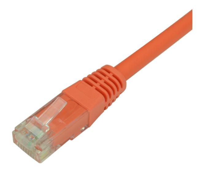
High Quality Cat 6 UTP Patch Lead Wired 258A (T568B) to 50 Micron Gold Plated RJ45 connectors. Each cable is supplied with fitted strain relief Boots for added protection. All cables up to 5m are made using standard core cable with cables over this length using solid core cable, which although not so flexible are more robust.
