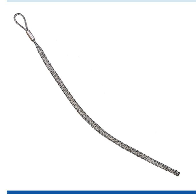
Consists of wire mesh tube with one pulling eye at one end. These grips are placed over the end of the cable, allowing the drawing in or recovery of cables.
