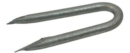
Galvanised steel staple, "U" shaped approximately 40mm wide and used to retain single strand suspension wire to poles when making a termination.
