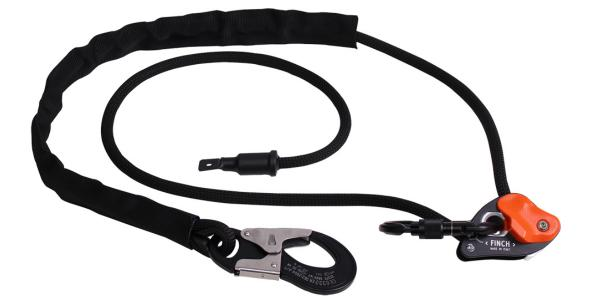
The RGP1 Finch can be used for work positioning by clipping onto both side D rings located on a work positioning belt and wrapping around a suitable structure, or as an adjustable restraint lanyard to prevent the user from entering the risk of a fall situation.
