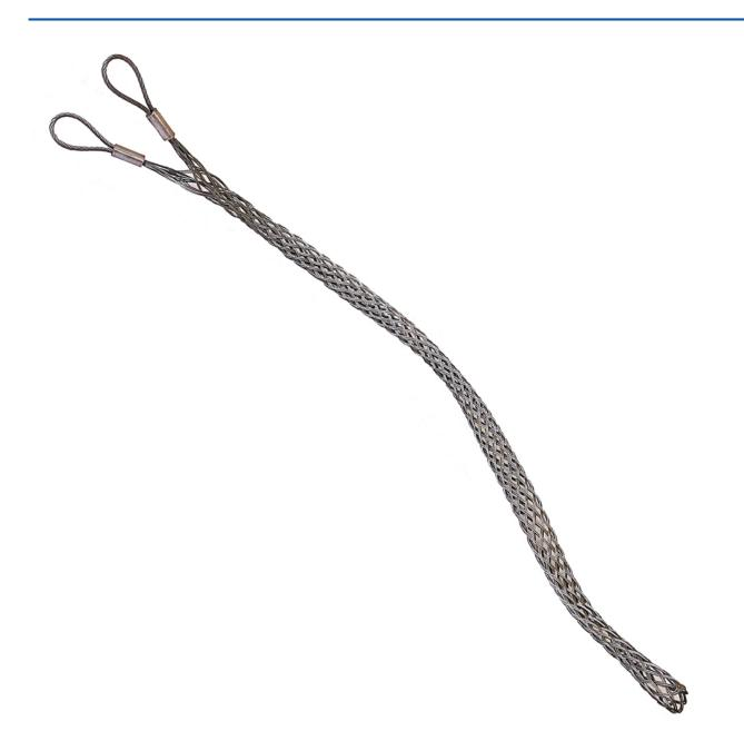
These fleeting eye cable grips have **double** pulling eyes. Unlike a standard single eye grip the eyes themselves are offset which means that you can have an opening in the weave on either end. This allows the cable to pass fully through it (providing there is no end termination of oversized fittings on it).
