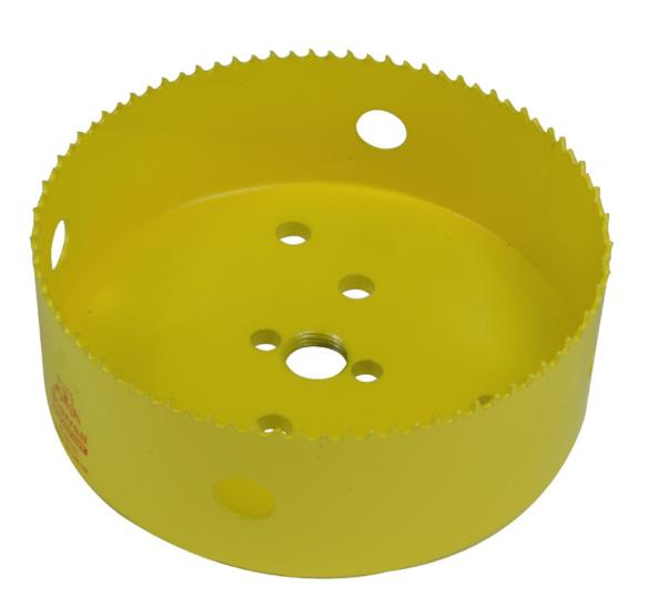
64mm (2 1/2 inch) Starrett Fast Cut Bi-Metal Holesaw with a cutting depth of 41mm. Requires arbor N76-1258 or N76-1260.
