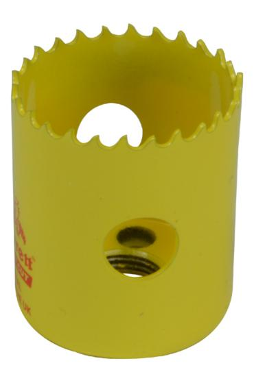
57mm (2 1/4 inch) Starrett Fast Cut Bi-Metal Holesaw with a cutting depth of 41mm. Requires arbor N76-1258 or N76-1260.
