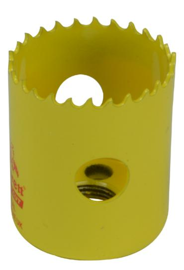
44mm (1 3/4 inch) Starrett Fast Cut Bi-Metal Holesaw with a cutting depth of 41mm. Requires arbor N76-1258 or N76-1260.
