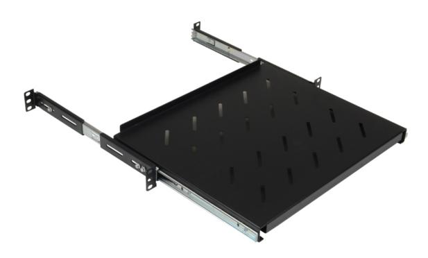
Fusion Contract Series sliding shelf is designed for use in 600mm deep cabinets. It has a depth of 350mm and extends out by 260mm.
