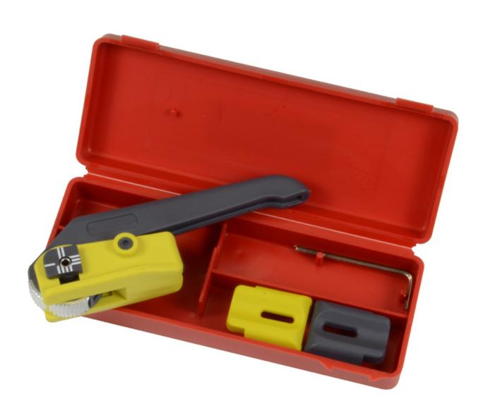
This 1A fibre stripper can be used to strip the sheath longitudinally from around the fibreflow microduct or other telco style cable without damaging it. The unwanted tube which surrounds the fibre can be stripped off with ease.
