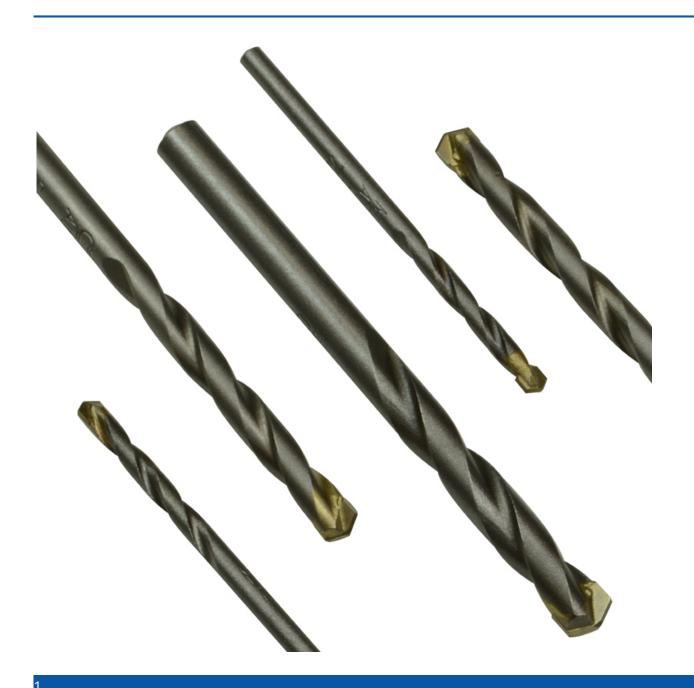
Tungsten carbide tip, long shank masonry drill bit with milled flutes for percussion and rotary drilling in concrete, brick and natural stone. DIN ISO 5468
