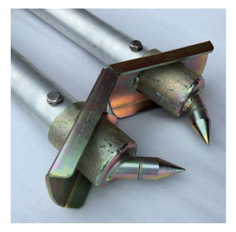
Designed to raise wood poles used in the construction of overhead power and telecom lines. This device is particularly useful in remote situations where vehicle-based methods of pole erection are impractical. Integral hand winch for raising pole lifting collar.
