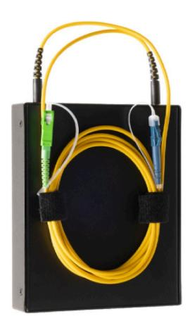
An OTDR requires a Launch Lead to be able to launch and receive test cable loss measurements for fibre optic links and reveals the insertion loss and reflectance of the near-end connection.
