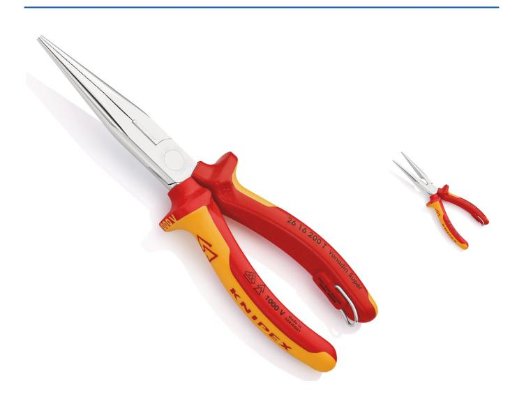
Handles insulated with multi-component grips, VDE-tested with integrated insulated tether attachment point for a tool tether. Elastic tips: dimensionally stable even when twisted Distortion-tolerant, elastic precision tips Half-round, long, tapered jaws With cutting edges for soft, medium-hard and hard wire Cutting edges additionally induction-hardened, cutting edge hardness approx. 61 HRC Cutting capacities medium hard wire (diameter) Ø 3.2 mm Cutting values hard wire (diameter) Ø 2.2 mm
