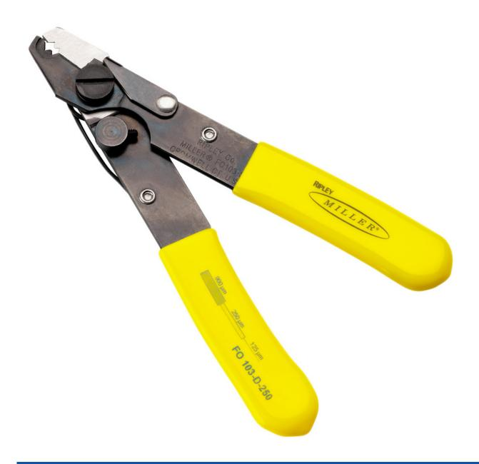
Two hole design efficiently strips away the 1.6 to 3 mm jacket or 900 micron tight buffer & 250 micron buffer coating from the 125 micron bare fibre in one compact tool that is factory-set & does not require any adjustment.
