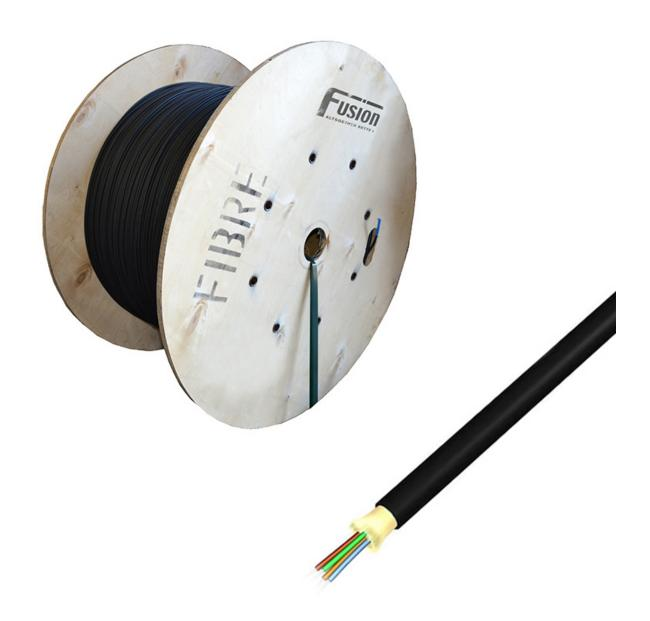
Universal tight buffer optical fibre cables have been designed specifically for internal and external applications. The outer jacket is water and moisture resistant, flame retardant, Low Smoke Zero Halogen.
