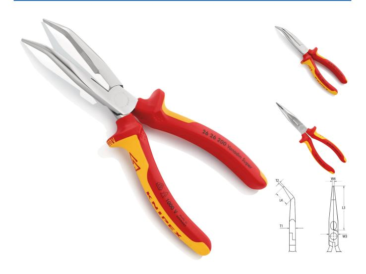
These forged, oil-hardened and insulated stork beak pliers with multi-component grip are ideal for installation, insertion and assembly, as well as powerful cutting. The cutting edges of the pliers are shaped to produce a pierced cut. The Knipex 26 26 200 also cuts hard wires.
