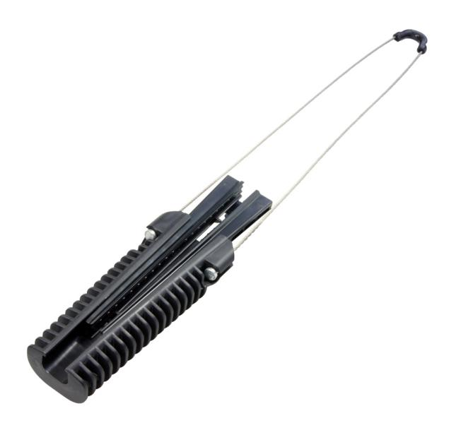
The ACADSS anchoring clamps present an open conical body, a jaw with two plastic wedges and a flexible bail. These cable clamps are used for the termination of fibre optic round ADSS cables deployed on distribution networks where spans do not exceed 90m.
