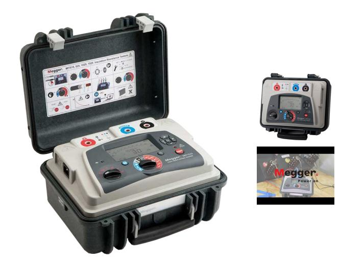
Offering CAT IV safety, the MIT1525 is compact, light 15 kV insulation resistance tester for the diagnostic testing and maintenance of high voltage electrical equipment. It benefits from the Megger dual case construction, Tough on the outside and fire retardant on the inside.
